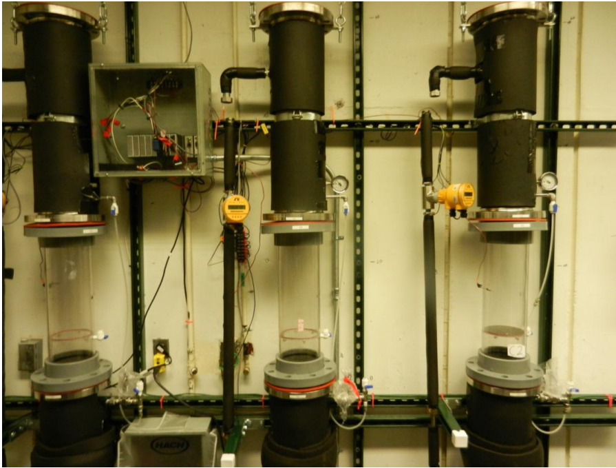
Figure 9. CHLE vertical strainer head loss columns [19]
