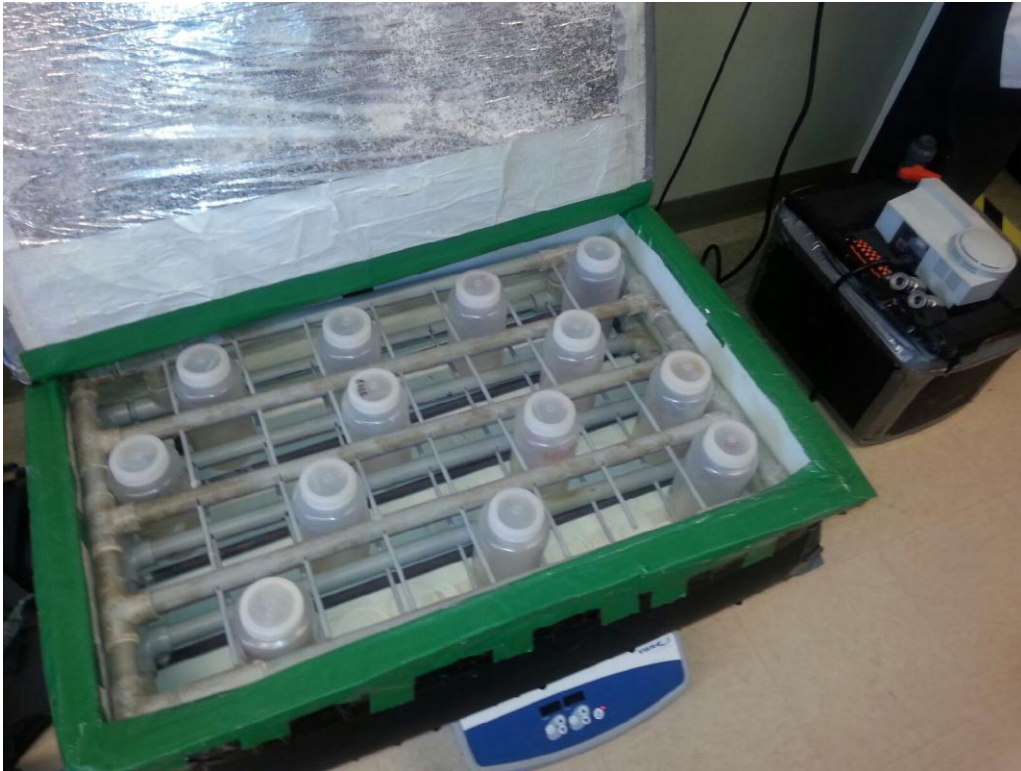
Figure 13. Hot bath with 1-liter Nalgene bottles
